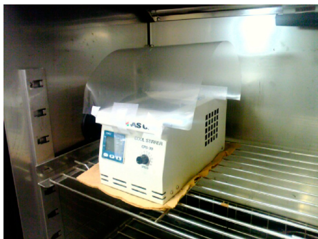
Figure 1. Image of the film-forming equipment with the cover in the thermo-hygrostat.
